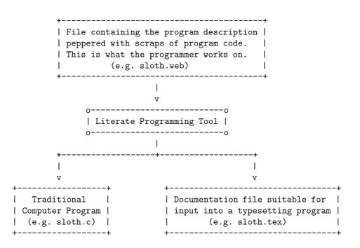
Literate programming tools could be organized in a number of ways. However, to fit in with current file and command line based environments, most tools conform to the traditional architecture shown here in which the user feeds in a file containing a literate program, and the literate programming utility generates program files and a documentation file.
