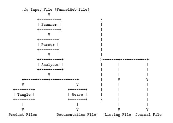
FunnelWeb processes each input file in a sequence of phases. If an error occurs during a phase, no subsequent phases are executed.
